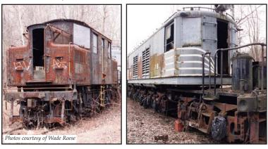
Rescue and restoration of two ex-NYC electric locomotives (1904 S1 *(above, left)* and 1926 T3a *(above, right)* motors)
