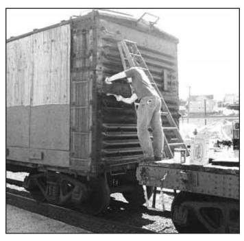
Rome applying rust stabilizer thathe A end with view of partly painted plywood.
