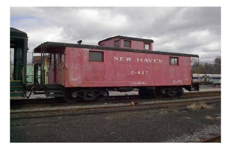
Arrived Danbury 4/96. Purchased from Berkshire Scenic Railway. Built May, 1944, by the Pullman Standard Co. First run on the New Haven RR, it was reconditioned in 1978 by Contrail. Restored to its "as-delivered" paint scheme by the DRM, it is still missing its roof-walk. Complete with stove, ice-box and toilet, it was a veritable apartment for the conductor, who might be assigned to the same freight-run with it for a number of months or longer.
