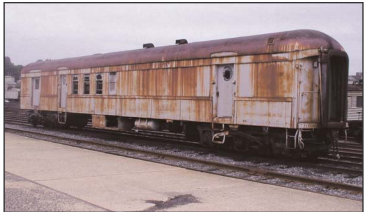
The RPO car as it stands in the railyard today. On its exterior work is needed mainly on the roof and windows. Then with a coat of paint covering those cosmetic rust stains, it will be an even more impressive looking piece.
