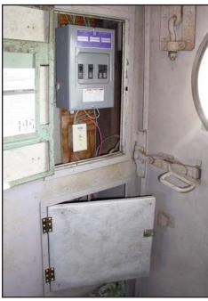
The newly installed circuit box. shown with its door open, is above a newly fabricated door which opens to other parts of the electrical panel. Below, Bill Britt works on removing a strip of the interior as he proceeds with restoration of the car. Having electric current also has enabled the car to be heated, which will allow work to continue during cold weather.
