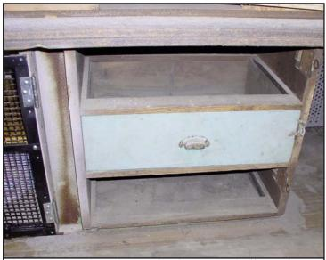
This appears to be a drawer for the personal effects of one of the crew of postal workers. It has the capability of being locked. Fortunately this drawer still remains as an example so that the remaining eight drawers are being fabricated using this one as an example. Elsewhere in the car there are hooks and space for hanging up the crew's outerwear.
