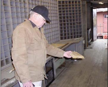
Bill Britt holds one of the "bolsters", showing the beveling on the 5-quarters thick piece of wood. He had to create the angle on the end by hand because of the unusual thickness. The new ones are evident in the lower photo. The third original one has the circular holes with the broken off ends of two missing tubes which extended to the ceiling. They helped keep the filled mail sacks from shifting. The "bolsters" apparently were used to keep the mail sacks off the RPO car floor.
