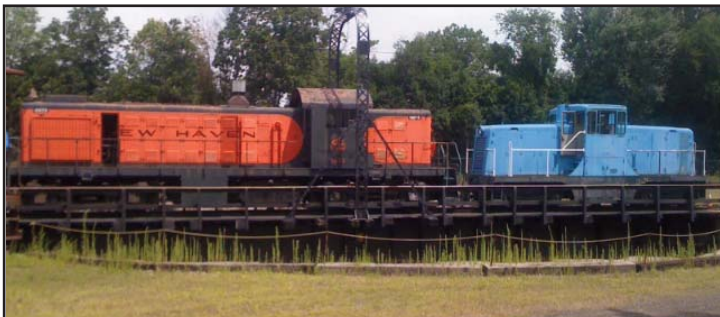
Bottom photo, taken by Chuck Sager, pictures the newly operating 44-tonner pushing the RS-1 across the turntable
