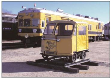
The DRM's #135 Sperry Rail Flaw Detection Car is seen behind a speeder on the center platform.
