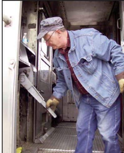
Above, setting the hand brake. Below, switching on/off the Budd car.
