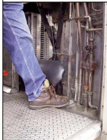
Above, blowing the air tank. Below, foot on the dead man's pedal of the RDC Budd car.
