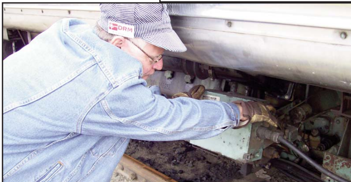
Above, setting the hand brake. Below, switching on/off the Budd car.
