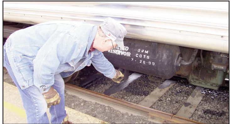
Above, blowing the air tank. Below, foot on the dead man's pedal of the RDC Budd car.
