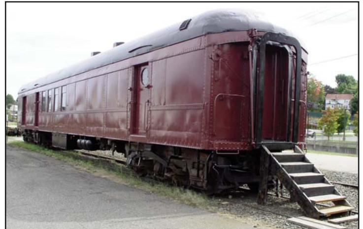
The RPO car's glossy epoxy coated black roof and Tuscan red sides have dramatically transformed the exterior of the car, making it a real eyecatcher!
