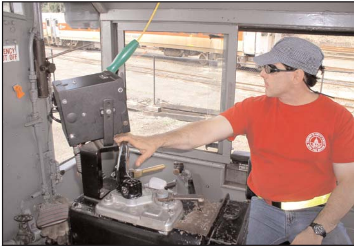
Engineer-trainee Jeremy Rice gives the RS1's throttle a tug, bringing the train back up track 18.
