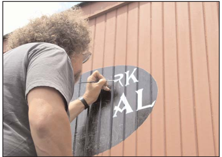
Ira begins the tedious process of hand-lettering each character by filling in the tracings he just made from a stencil.
