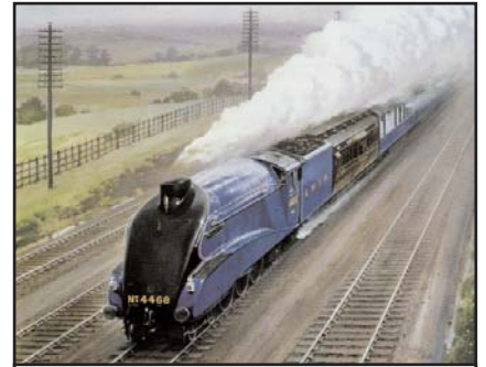
The ultimate record for a steam locomotive is held by the London&Eastern's No. 4468, Mallard, an A4 class 4-6-2 designed by Sir Nigel Gresley. It attained a speed of 125 mph pulling 240 tons over a course of five miles on July 3, 1938. Illustration courtesy of The Science Museum, London.
