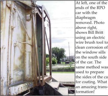
ends of the RPO car with the diaphragm removed. Photo above right, shows Bill Britt using an electric wire brush tool to clean corrosion off the window sills on the south side of the car. The same method was used to prepare the sides of the car for coating. What an amazing transformation!
