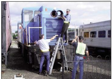
Dan Carleton gets ready to hand Jim Teer (left) part of the fixture he has just removed that was holding the headlight for one of the 44 tonners. Jeremy Rice stands ready to assist. Dan proceeded to scrape away corrosion from the socket. The removed portion is corroded but will serve as a model for a newly fabricated piece.
